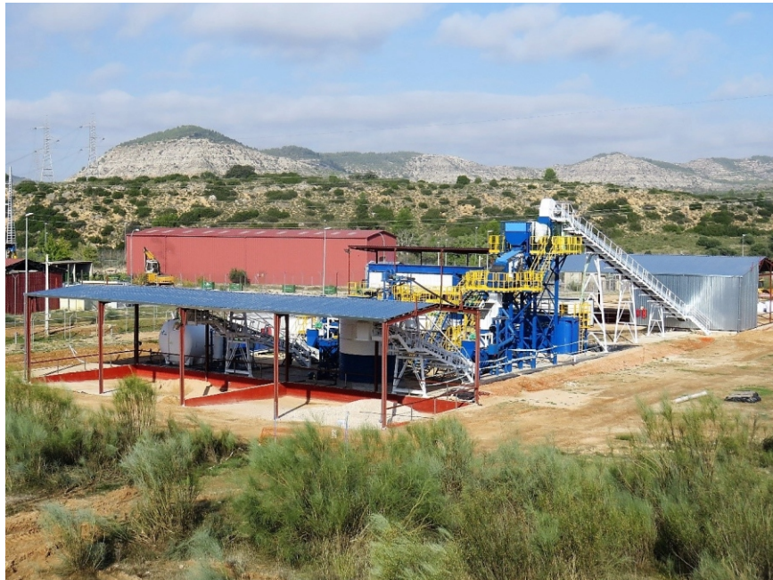
Image of the soils treatment plant at the José Cabrera nuclear power plant.
