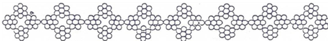
Figura 4: Cable plano 8 (4 x 7 +1)
