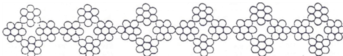
Figura 3: Cable plano 6 (4 x 7 + 1)
