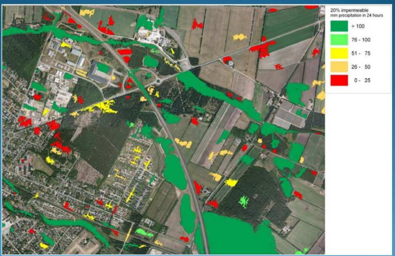
Análisis de sensibilidad a la Iluvia, con la hipótesis de 20% de impermeabilidad del terreno. Fuente: The Blue Spot Model- development of a screening method to assess flood risk on national roads and highway systems. Report 3. May 2010
