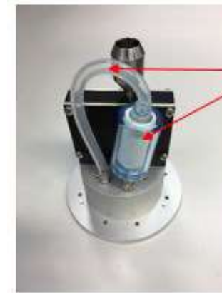
Filter of the Laser Particulate Counter
