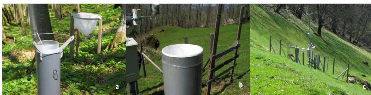
Figure 5-1: Throughfall (a) and open-field (b, c) collectors for rain in summer (a) and for snow in winter (b) in the northern Alps, Switzerland (Image: WSL)
