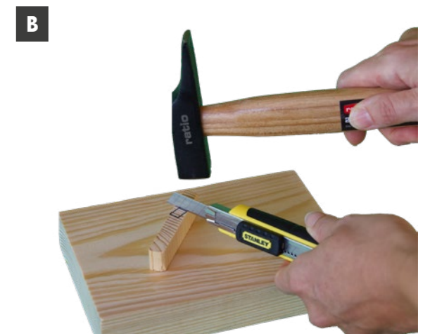
Obtain the 15x15 mm piece using a utility knife and a hammer.
