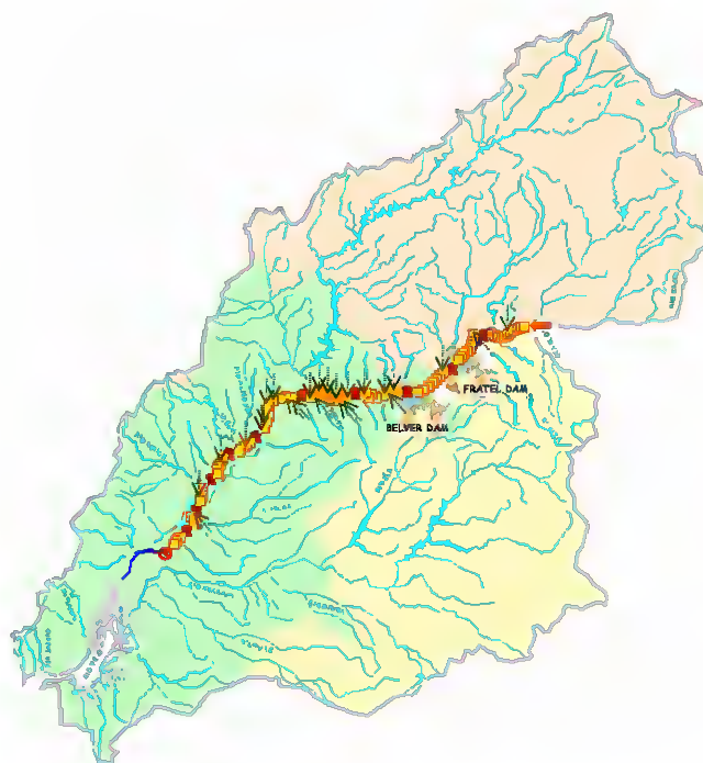
Figure 1 - Reaches, computational elements and 25 point loads considered, and localisation of the dams.
